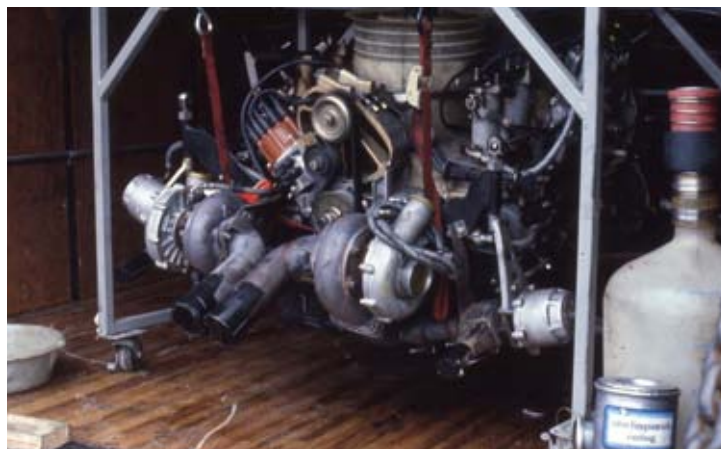
TWIN TURBOS bristle from the rear of this spare racing engine. The dark grey color is the exhaust side. The light colored side is the intake.
