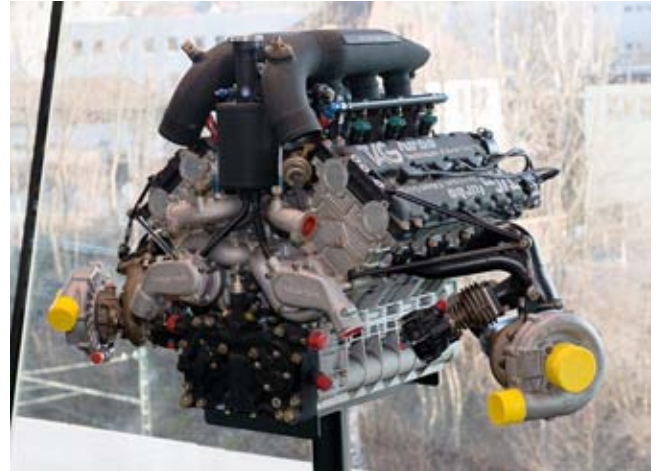
The TAG-Porsche Formula 1 engine as used in the McLaren MP4/2. The Turbos (with yellow caps on the intake side) connect to air-to air intercoolers in the car which, in turn connect to the black intake plenums at the top of the motor. Displacing a mere 1500 cubic centimeters, this little V-6 engine ultimately produced 960 hp. in qualifying tune. Photo from Wikicommons.
