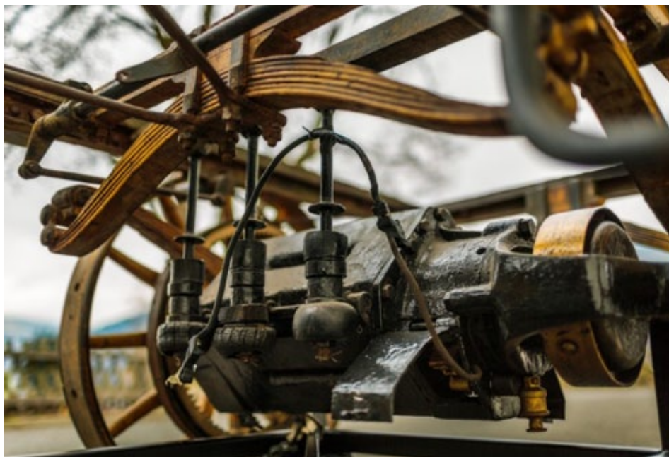
Above: The P1's motor; below: Ferdinand Porsche stamped the major components "P1."
