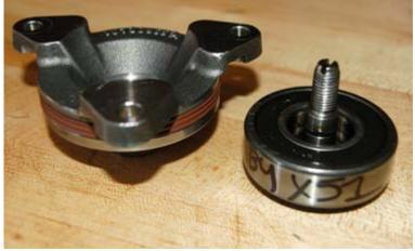
Some late model year 2005 engines were fitted with a larger bearing that is not serviceable without a complete teardown of the engine.
