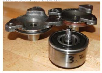
MY02-05 will need a single row Retrofit™ kit, identified by a narrower single row ball-bearing and wider IMS flange.
