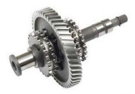
The purpose of the intermediate shaft is to drive the camshafts indirectly off the crankshaft. By using an intermediate shaft, the speed of the chains are reduced, which is better for chain life. This basic design was used throughout the entire lifespan of the aircooled six-cylinder Mezger engine used through 1998. The inclusion of an intermediate shaft which drives the camshafts indirectly off the crankshaft has been a mainstay of the horizontally-opposed flat 6 engine utilized by Porsche.
