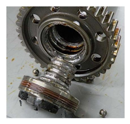
By far, the single row ball-bearing used starting in model year 2000 through 2005 are the most problematic. Based off projections calculated by a fellow Porsche enthusiast and retired bearing engineer from Timken, they figure a 90% survival rate of the single-row 6204 ball-bearing used in the IMS at 90,000 miles\* – resulting in a staggering 10% failure rate (called the LIO life)!
