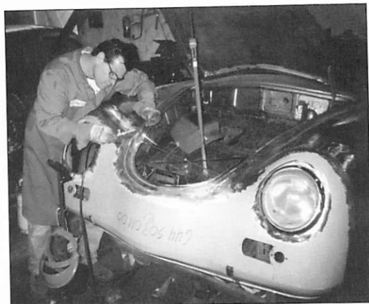
Jim installing a factory Speedster nose clip
