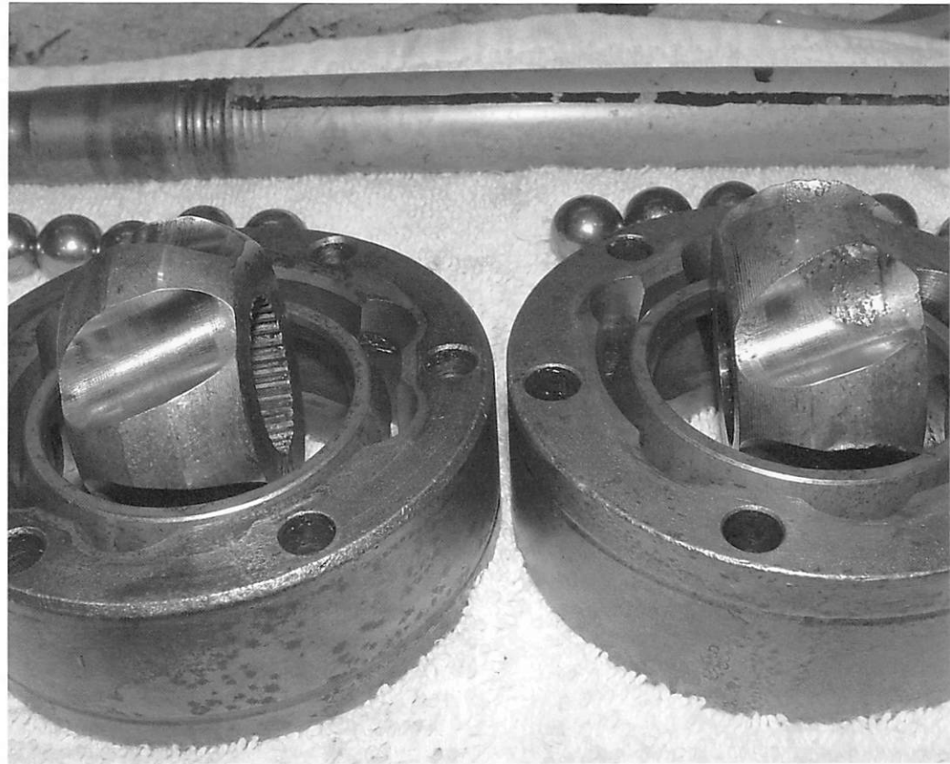
The 944's worn CV joints. Notice the wear in the cups, especially visible on the right-most joint.
