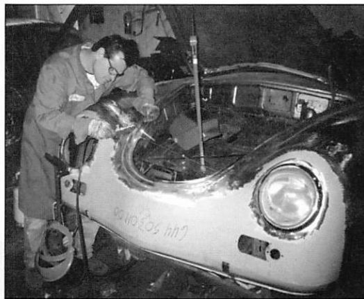
Jim installing a factory Speedster nose clip
