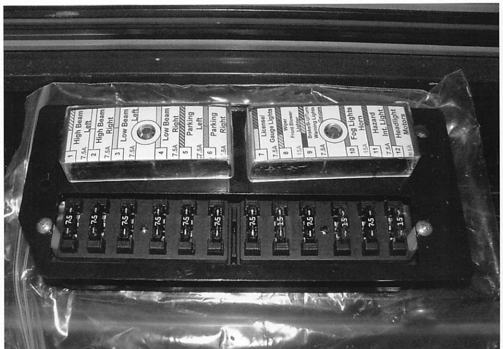
Below: A new blade-type fuse box for the 914 will enable fast getaways.
