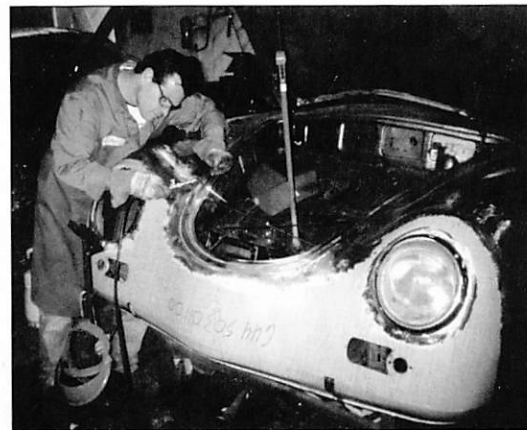
Jim installing a factory Speedster nose clip
