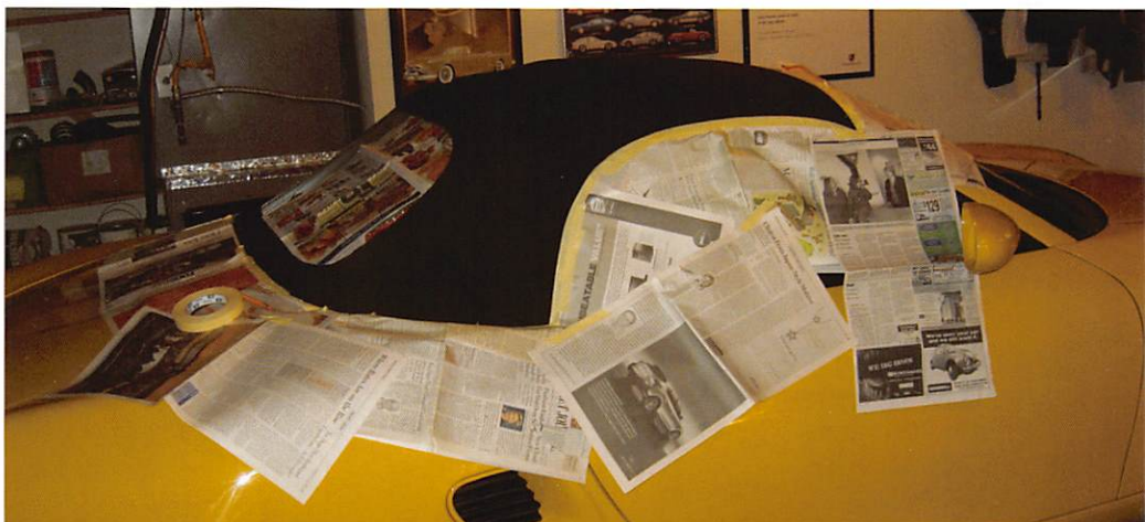
Above: Mask well and spray. Below: The proof is in the beading.
