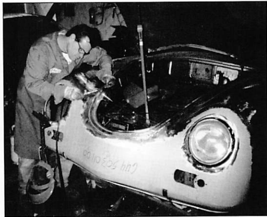
Jim installing a factory Speedster nose clip
