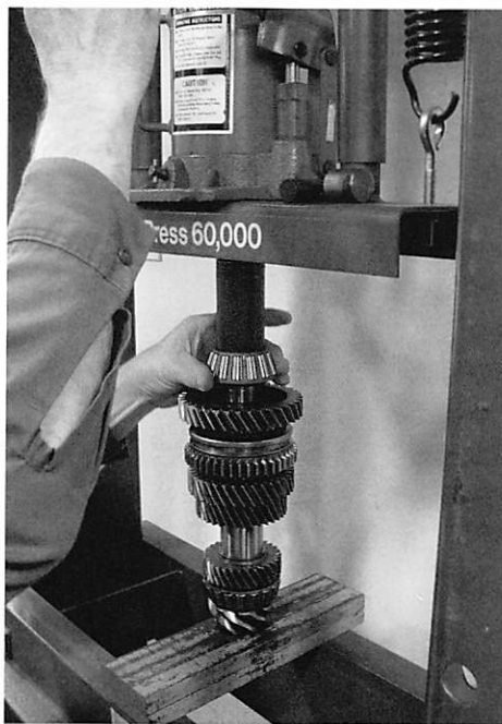
Photo 1: 944 gear clusters getting reacquainted in a 60-ton hydraulic press.
