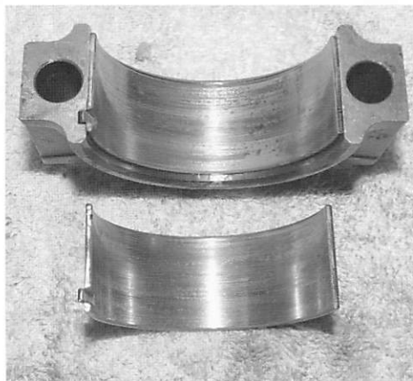
Photo 1: The result of a loss of oil pressure.
