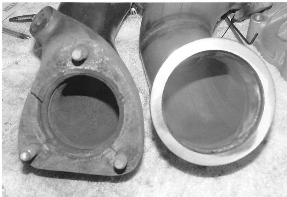
Photo 2: The cracked turbo downpipe alongside its replacement.
