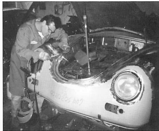
Jim installing a factory Speedster nose clip
