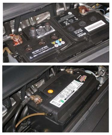
Top: Lead acid battery – 3 cells open to add water. Overflow hose on left end. Above: Sealed lead acid battery.
