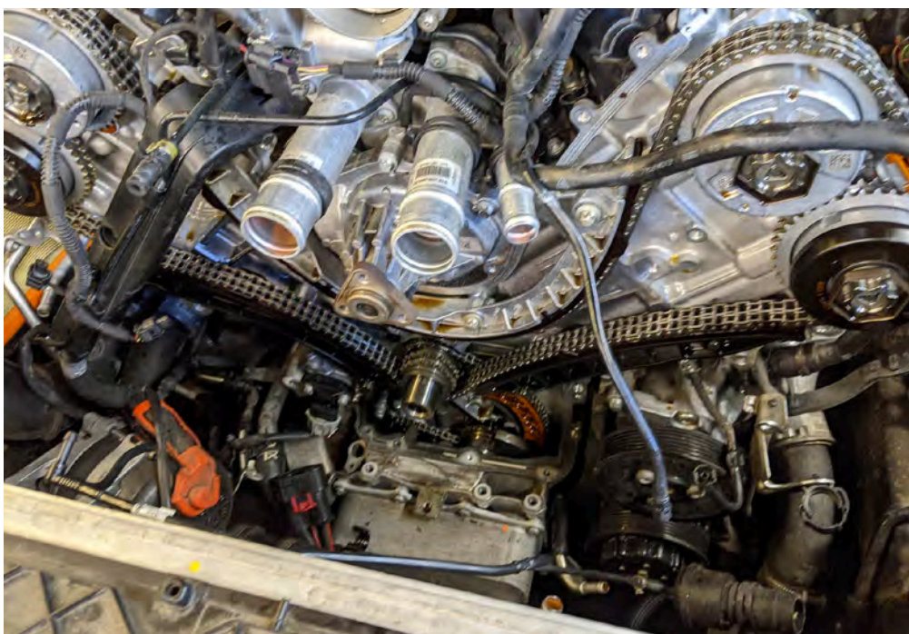
Left: Oil drips. Above: Cayenne V6 timing cover leak repair.
